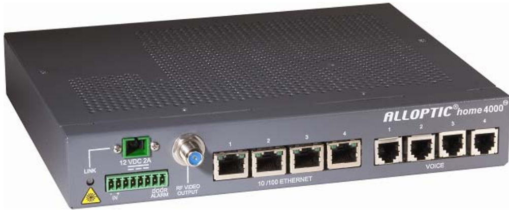
Figure 7 – Photo of an ONT. Over 4,000 of these units are already deployed in Australia (Source: Opticomm)
